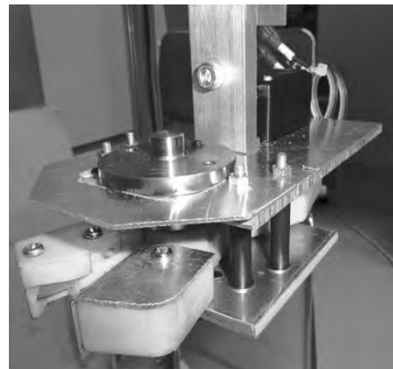
Fig.5 Line cut unit.
