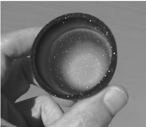
Fig.3 Photograph showing the alumina crucible with ruby layer.
