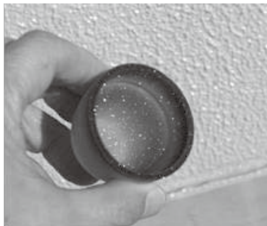
Fig.3 Photograph showing the alumina crucible covered with ruby thin film.
