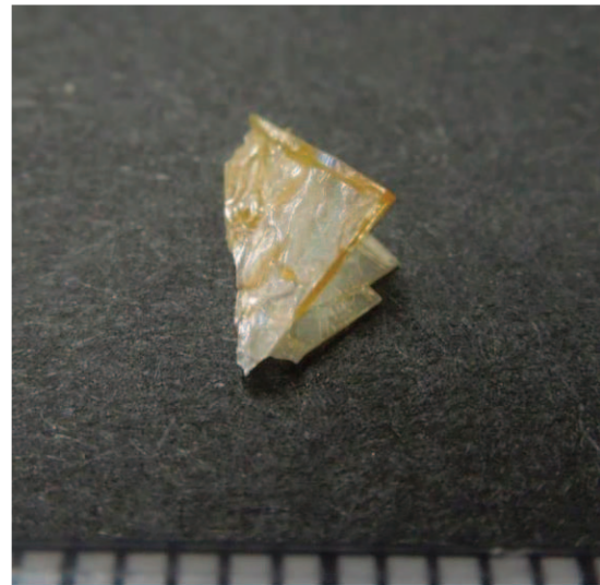
Fig.4 Grown butterfly twin of BaTiO 3 .
