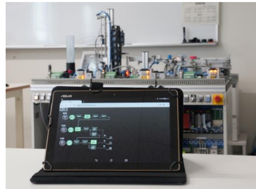
Fig.3 Remote monitoring via Ethernet.
