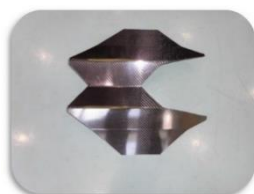
Fig.7 CFRP molding by autoclave
